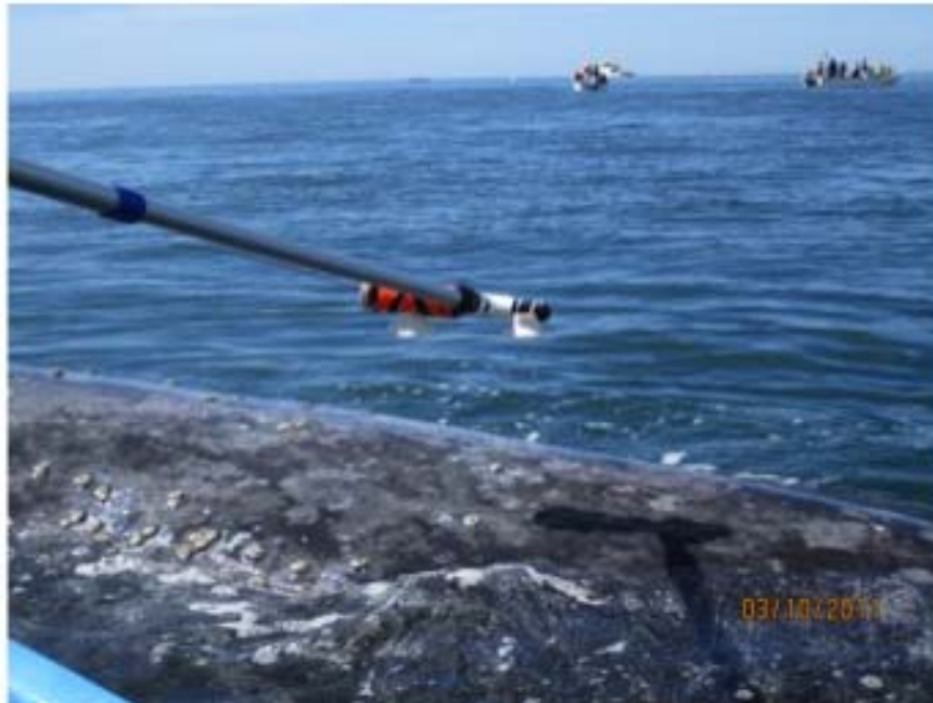
Figure 4. B-Probe tag assembly (with orange floatation device and white suction cups) attached to the deployment pole prior to tagging the adult gray whale. (dgreb_0160)
