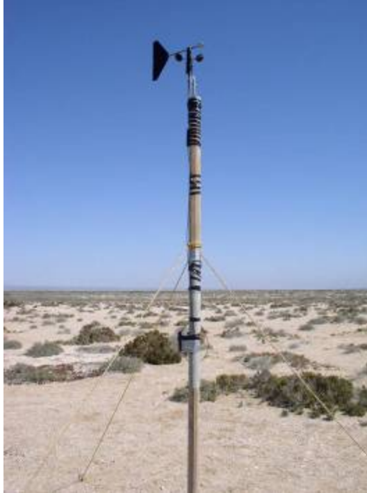
Figure 8. HOBO wind station sampling direction and speed at Punta Piedra
