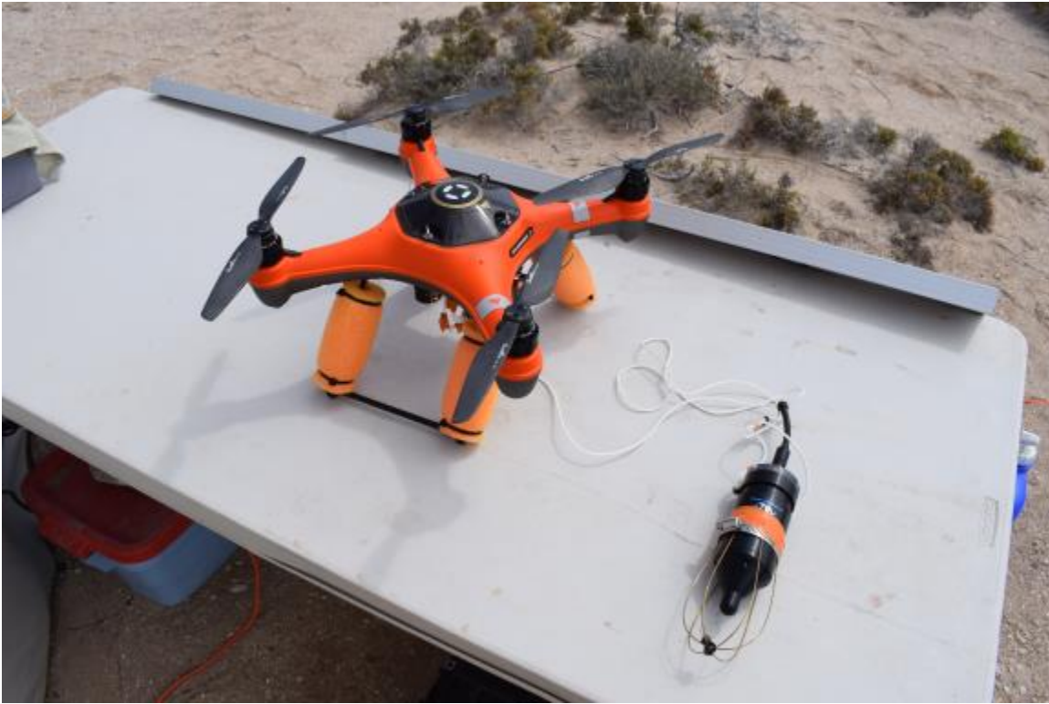
Figure 4 – Swellpro SplashDrone 3+ with hanging SoundTrap 300STD.
