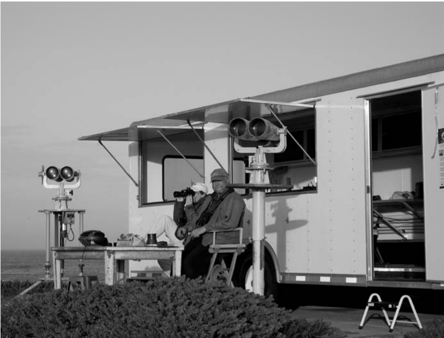
Figure 2. Observer station including mounted 25X binoculars for search to the horizon offshore and hand-held binoculars for tracking animals near shore.
